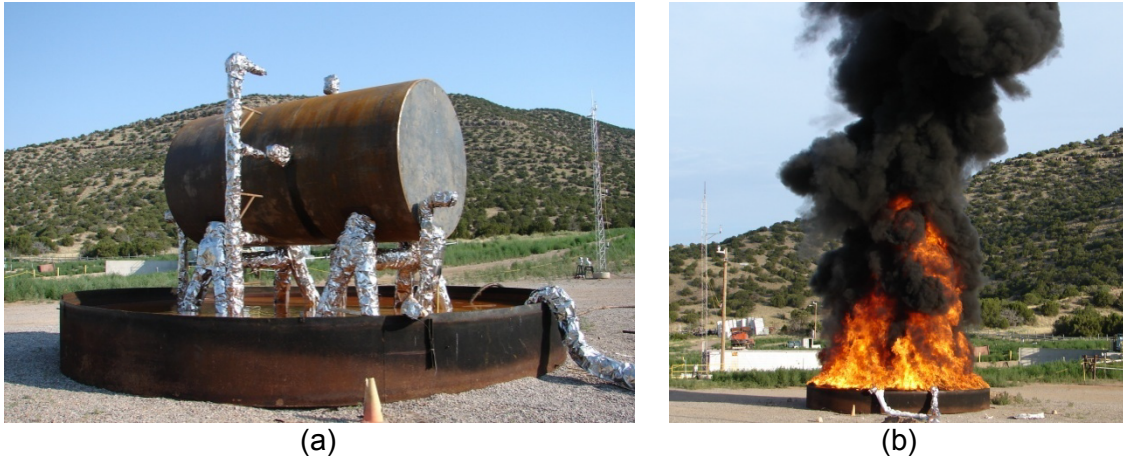
Figure D-29 Large calorimeter fire test: (a) test setup and (b) fire fully engulfing the calorimeter
